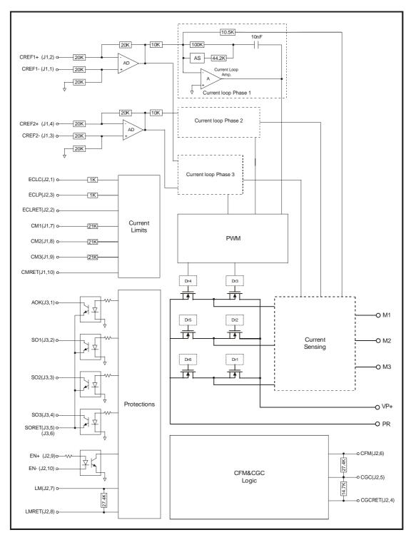
Figure 2-1: Raven Block Diagram
